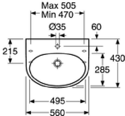
Mounted with flexible bracket dimensions, bracket length 260 mm. Can also be mounted directly on wall with bolts, required when mounting together with bathroom cabinet A659. Bolt projection from finished wall must be  $50 \pm 2$  mm. Brackets and other fasteners not included.
