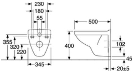
Intended for installation with our Triomont fixtures. Mounted with bolts directly on the wall. Washers, bushings and nuts (M12) included, but not bolts (included with Triomont fixture). Bolt projection from finished wall must be  $60 \pm 2$  mm. See included installation instructions.
