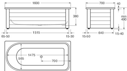
Bath panel for full or half bath panel delivered with end panels preinstalled. Front panel and concealed profile are then assembled into a frame. The frame is adjusted horizontally with the adjustable feet. The bathtub, which is equipped with damping/friction material under the corners, is lowered into the frame. The plastic drainpipe is cut and connected to the floor drain. Installation instructions are included.
