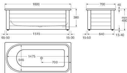
Bath panel for full or half bath panel delivered with end panels preinstalled. Front panel and concealed profile are then assembled into a frame. The frame is adjusted horizontally with the adjustable feet. The bathtub, which is equipped with damping/friction material under the corners, is lowered into the frame. The plastic drainpipe is cut and connected to the floor drain. Installation instructions are included.
