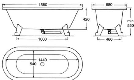
The four feet are mounted with two bolts on the welded brackets on the bottom of the tub. The plastic drainpipe is cut and connected to the floor drain. Level the bathtub horizontally with the adjustable feet (adjustable to 25 mm).
